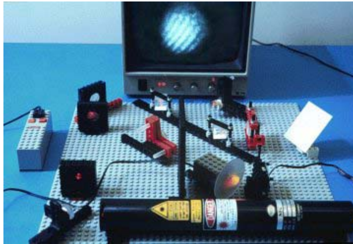
Fig. 16. Mach-Zehnder interferometer. Two fringe patterns are formed, one on the screen on the right and another on the rotating ground glass imaged by the ccd camera, as shown in the monitor.
